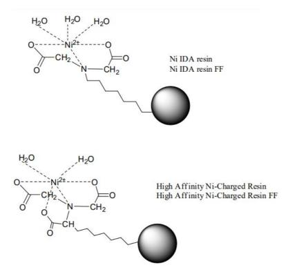
Figure 1. Schematic diagram of the chemical structure of Ni IDA Resin, Ni IDA Resin FF, Hi affinity Ni-Charged Resin and Hi affinity Ni-Charged Resin FF
